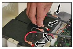
**3** Detach the battery cables from the four battery terminals.
